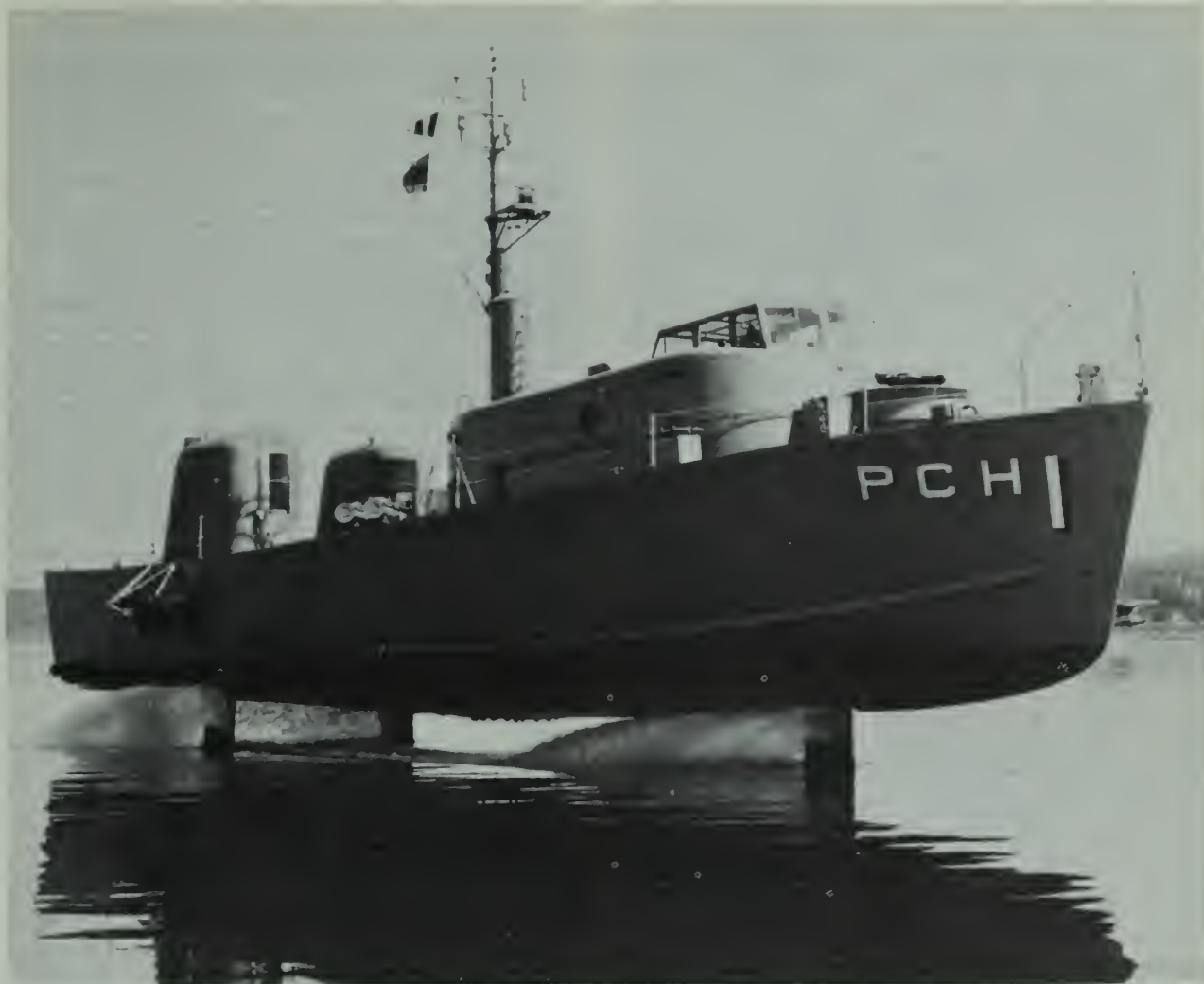
USS High Point (PCH-1)—Notice space between bottom of her hull and surface of the water.
